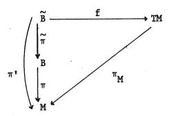
In local coordinates x for M, (x,u) for B (u for the inputs) and (x,u,q) for  $\widetilde{B}$  (q for the disturbances) this definition simple comes down to  $\dot{x} = f(x,u,q)$ .
